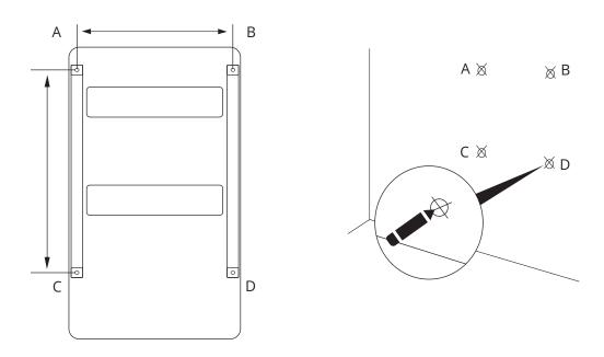
3. Using an 8mm drill bit, drill into the wall where you marked them out in step 2).
